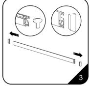
3.Remove the plastic end caps from the top snap bar there are two kinds of snap bar. changed according to diffevent items.
