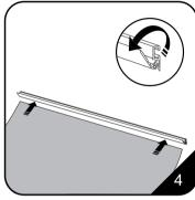
4. Open the snap bar then insert the top edge of the graphic.
