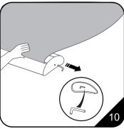
10. Activate the spring tension by removing the Allen Key. Pull the Allen Key while holding on to the attached graphic. Save the key in the side cover
