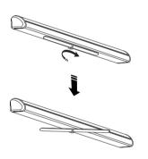
Underneath the base unit is one foot stand, to enable this, tilt the unit backwards and turn the two feet stands to a  $90^\circ$  from the base. This keeps the body standing.
