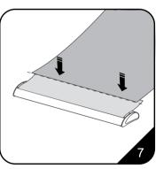
7. Peel off the adhesive paper along the edge of the base's leader roll and attach the bottom transparent adhesive tape at least 4cm wide of the banner. Make sure the banner is straight. both sides.
