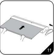
11.Carefully allow the graphic to recoil into the base unit, then reattach the chrome covers. the round end belongs to the bottom base.
