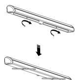
Underneath the base unit are two feet stands, to enable this, tilt the unit backwards and turn the two feet stands to a  $90^\circ$  from the base. This keeps the body standing.
