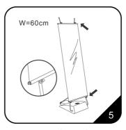
7.The graphic can be firmed by fixing the snap rail on the framework,as the pic. then completed.
