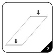
3.Attach a 4cm wide transparent plastic piece on the top and down of the graphic' back in order to strengthen it.
