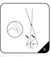
5.Fix the 2 small poles into the holes on the X poles, as the pic showing.
