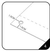
4. Punch in the 4 angles of the graphic, then fix the special rings in it, as the pic showing.
